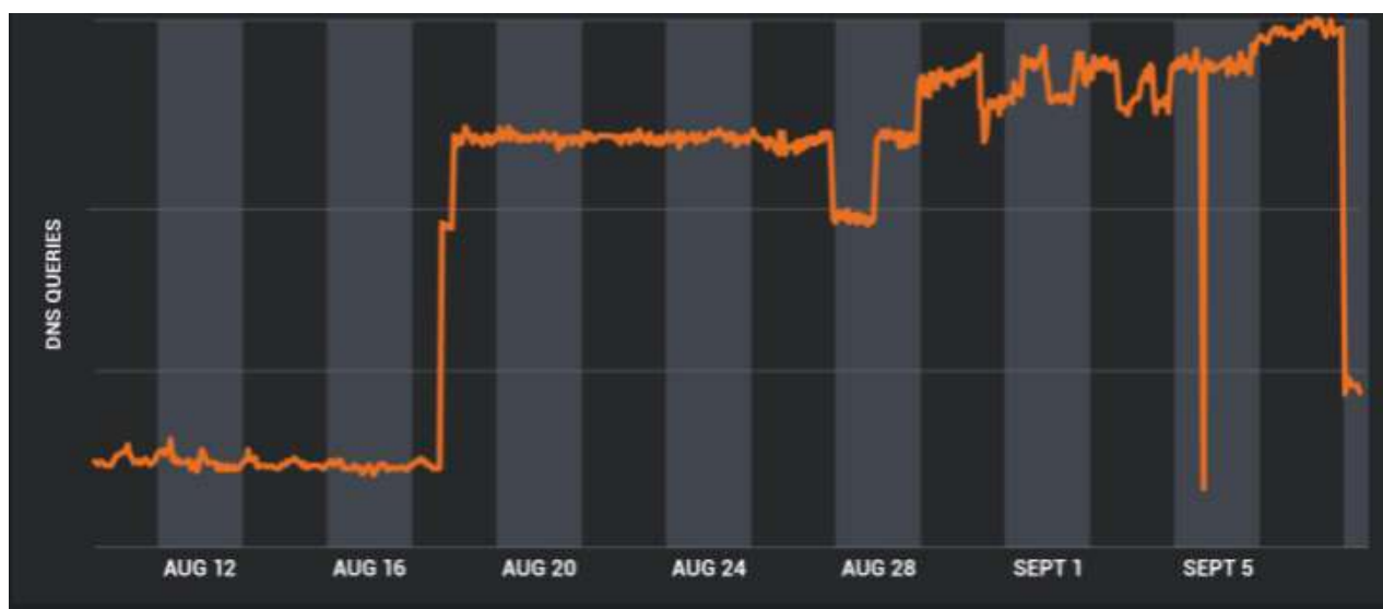
Fig 1 – DNS requests activity increasing to the t.amynx.com C2 server
